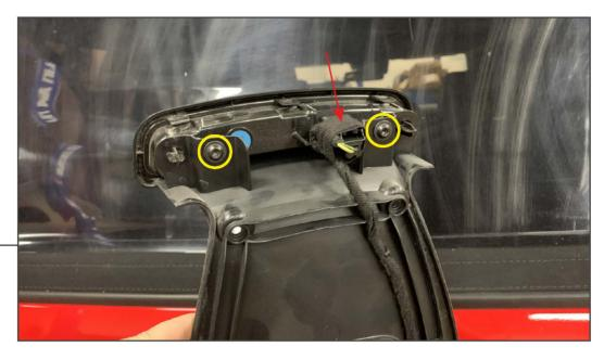
Unplug the vehicle third brake light. Then, remove (2) T-25 Torx screws from the third brake light and remove from the vehicle.
