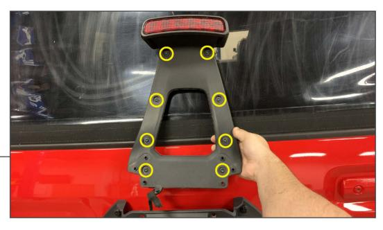
Lift the brake light housing upwards, and remove (8) T-25 Torx screws from the light housing.
