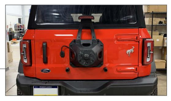
Remove the vehicle spare tire from the tailgate tire carrier using a lug wrench.
