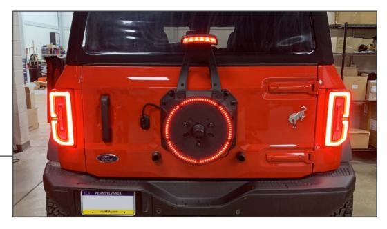
Fit the spare tire brake light to the vehicle tire carrier. Plug the spare tire brake light into the previously routed harness from the above tire brake light.
