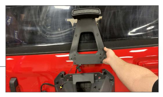
Assemble the brake light housing using the original (8) T-25 Torx screws. Ensure the wiring harness are not interfering with the housing assembly. Moderate force may be necessary to seat all areas of the housing.
