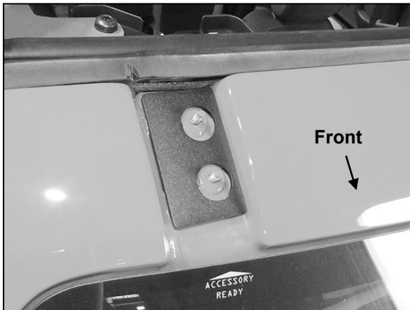
(Fig 5) Place Bracket Shim over threaded studs
