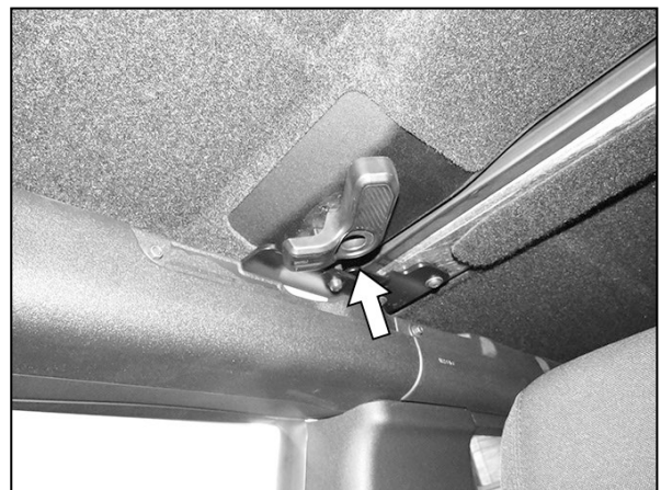
(Fig 22) If necessary, loosen screw 2-3 turns to adjust and fasten latch (arrow)
