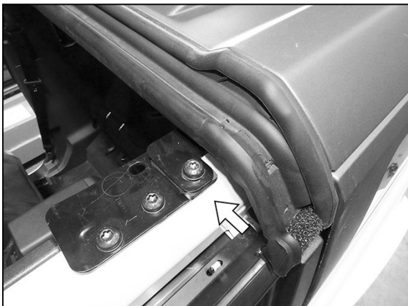
(Fig 21) Top Roof Spacer installed between top bracket (arrow) and inner roll bar (driver/left side pictured)
