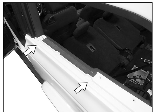
(Fig 14) Remove backing and apply driver/left adhesive backed Foam Side Seal to top of body (arrows)
