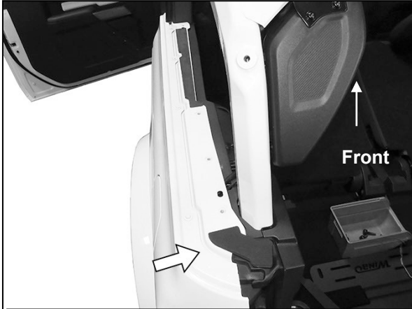
(Fig 15) Apply adhesive backed Foam Rear Seal to top of body
