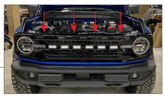
Secure the top of the grille to the radiator support using the original (4) 10mm bolts. Tighten until secure.
