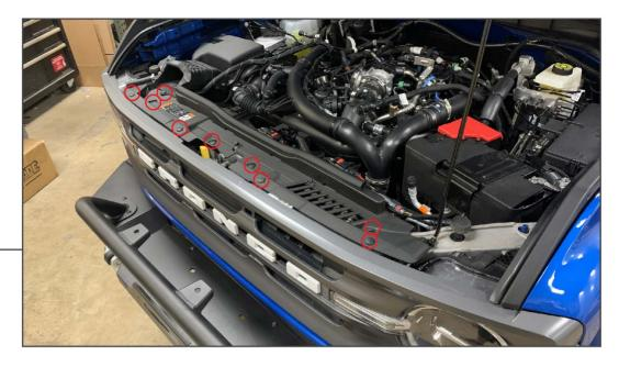
Open the vehicle hood. Remove (9) plastic push clips from the upper plastic trim. Remove the trim panel from the vehicle.
