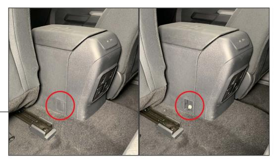
Locate the rear center console bolt covers on each side of the center console. Remove the covers using a plastic pry tool. Locate and remove the (1) 7mm bolt from each side of the center console.
