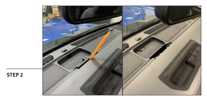
Using the provided plastic trim panel tool, pry the "ACCESSORY READY" panel from the vehicle dashboard.
