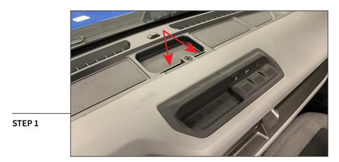
Remove (2) T-20 Torx screws from the "ACCESSORY READY" panel in the dashboard.
