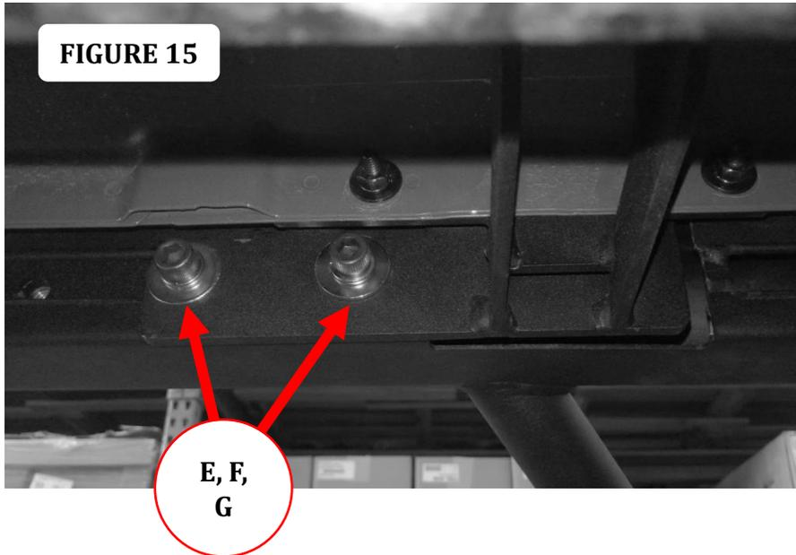
**Step-10** Align the Dominator running board with the vehicle and tighten all bolts securing the running board to the front, center and rear brackets. Repeat the above steps to install the driver side running board. Remember to check and retighten the nuts and bolts every six months.
