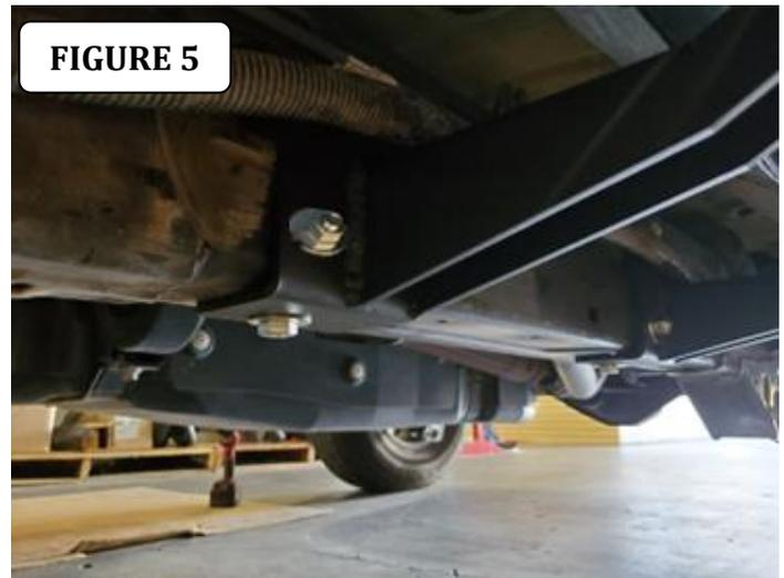
**Step-4** At the rear location, locate the threaded hole on the bottom of the frame and the slotted hole. Introduce a ½" bolt plate into the obround hole, use a vinyl gasket to prevent the bolt plate from falling into the frame rail. Secure the rear bracket to the bolt plate using (1) ½" flat, (1) ½" lock washer and (1) ½" hex nut. Secure the bottom hole using and (1) M12 hex bolt, (1) ½" flat washer and (1) ½" lock washer. Figure 7. Leave the bolt and nut loose for final adjustment.
