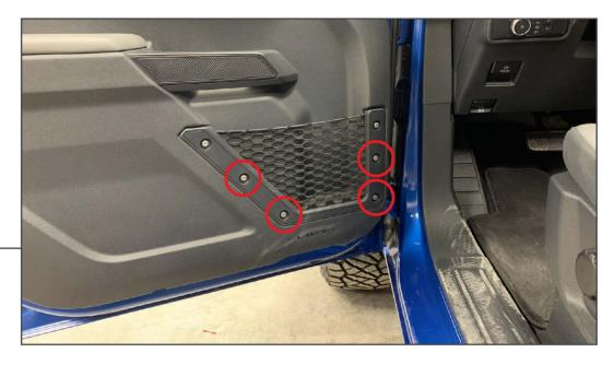
Remove (4) T-30 Torx bolts from the vehicle door storage net.
