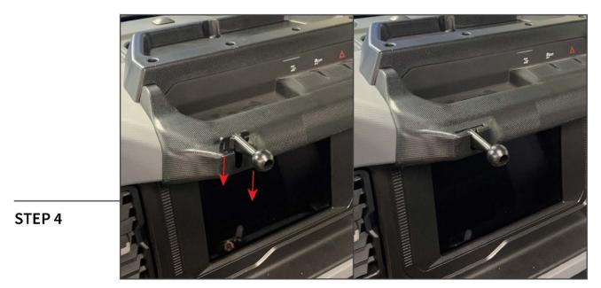
Press the (1) ball mount into the storage organizer assembly. The mount will audibly click into place when secure.
