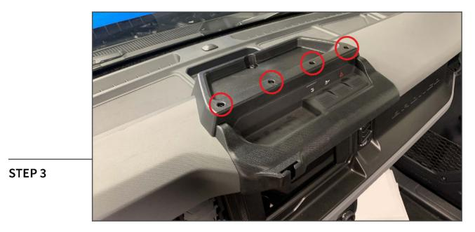
Tighten the (4) small Allen bolts until secure.
