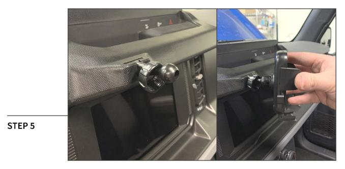
Fit the nut from the back-side of the phone mount onto the ball mount. Then, press the phone mount onto the ball mount. Thread the nut onto the phone mount. Adjust the phone mount to the desired position, and tighten the nut to lock the phone mount into place.
