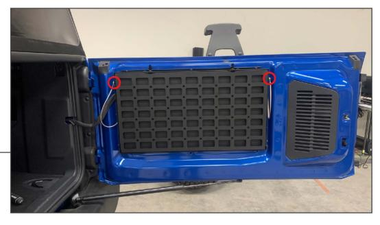
Fit the molle panel into the bottom of the tailgate table. Then, secure the hanging straps to the bottom of the tray using (1) M6 x 15mm Allen bolt and (1) M6 flat washer.
