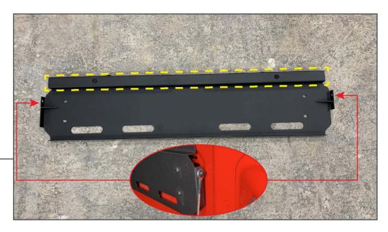
Install (1) foam strip on the upper and lower mounting plates to prevent the plates from directly touching the vehicle paint.
