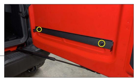
Mount the lower mounting plate to the vehicle tailgate using (2) M6 x 25mm Hex bolts, (2) M6 lock washers, (2) M6 flat washers, and (2) M6 threaded inserts. Fits the inserts into the lower tailgate slots, then tighten the bolts. Tighten until secure.
