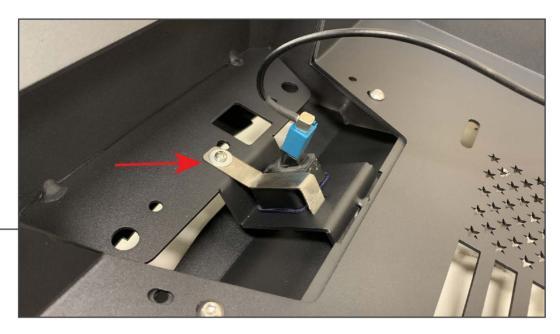
Place the tailgate panel on a soft surface face down. Remove (1) Phillips screw to move the bracket away from the camera mounting hole. Fit the camera into the mounting hole, ensuring the orientation is correct. Re-place the bracket over the camera, and tighten the Phillips screw until the camera is secure.
