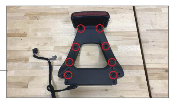
Remove (8) T-25 Torx bolts from the third brake light to reveal the third brake light wiring/bolts.
