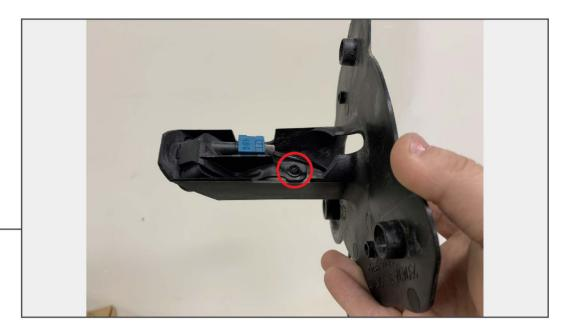
Remove (1) T-20 Torx bolt to remove the camera assembly from the housing. Set the camera aside for installation later.
