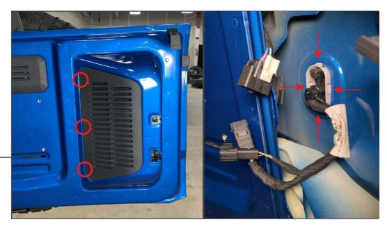
Open the vehicle tailgate and remove the plastic cover panel by dislodging the (3) metal clips using a panel removal tool. Unplug the (2) electrical connectors for the backup camera and brake light. Press the plastic tabs on the tailgate grommet to route the wiring harnesses outside the vehicle door.
