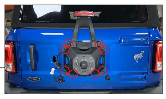
Remove (8) 13mm bolts to remove the spare tire carrier assembly from the vehicle tailgate.
