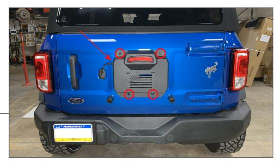
Route the wiring harness through the notch on the LH side of the panel. Then, secure the panel to the vehicle tailgate using (4) original 13mm bolts. Plug the wiring harness grommet into the tailgate.
