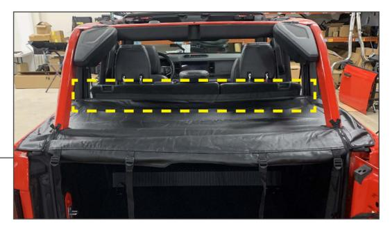
Press the Velcro at the front of the tonneau cover to the vehicle rear seats. The Velcro will attach to the vehicle rear seat material.
