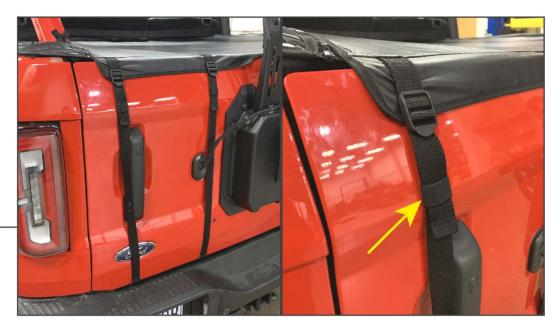
Close the vehicle taiglate. Route the (4) rear tonneau cover straps over the top of the tailgate. Clip the strap hooks to the bottom lip of the tailgate. Tighten the straps evenly to add tension to the tonneau cover. Fit the strap after tightening into the pre-installed elastic strap holder.
