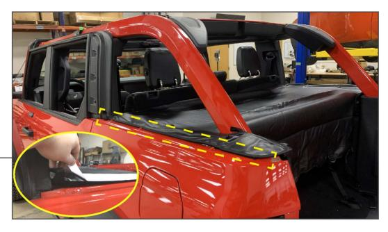
With all bolts started, peel the tape backing from the Velcro, and adhere the Velcro strip to the vehicle body on both sides.
