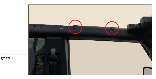
Remove (2) 8mm bolts from the vehicle roll bar above the rear seats.
