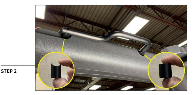
Using the (1) concave spacer and (1) cylinderical spacer, align the grab handle to the vehicle. Secure the grab handle to the vehicle using (2) M6 Allen bolts into the original vehicle bolt holes.
