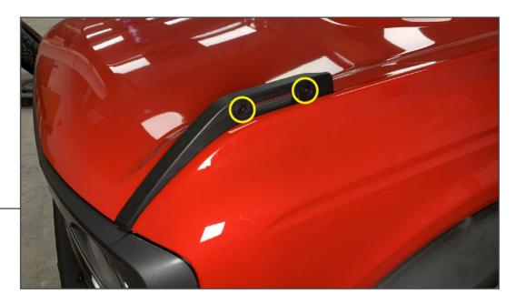
Locate the fender mounted accessory mounting point. Remove the (2) T-30 Torx bolts in the accessory mount, but do not remove the threaded insert. The threaded insert will be reused.
