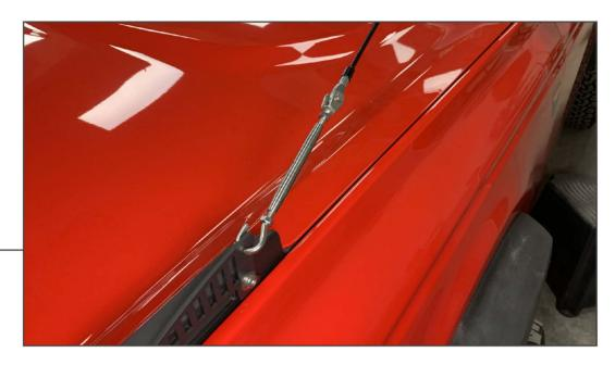
Secure the adjuster assembly to the limb riser cable by pinning the cable eyelet through the adjuster assembly pin. Then, loosen the adjuster and hook the front hook into the previously mounted fender mounting bracket.
