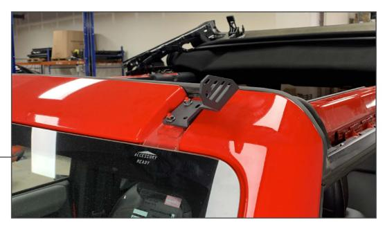
Align the appropriate windshield mounting bracket to the vehicle, take note to the direction of the outside of the mount to identify each side. Then, secure the mount into place using the original (2) 10mm nuts.
