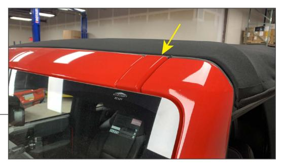
Locate the "Accessory Ready" panel above the windshield. Remove the cover by pressing the release tab and pulling the cover away.
