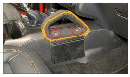
Install the accessory mount with the storage bag to the vehicle, and secure into place using the original (2) T-30 Torx bolts. Tighten the hardware until secure, do not over-tighten.
