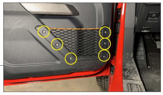
Remove (6) T-30 Torx bolts from the vehicle door panel.
