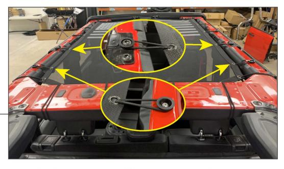
Begin to secure the rear sides of the mesh top using (4) small elastic bands [without hooks].
