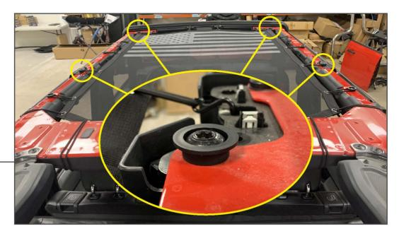
Remove the OEM (4) T-50 Torx bolts from the top retainer brackets. Fit (1) provided plastic washer onto the bolt hole, and then re-install the original Torx bolts. The washer will be used to fit the elastic straps around.
