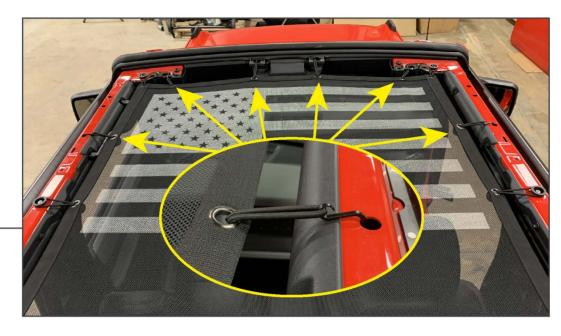
Begin securing the front of the mesh top to the vehicle roll bars using (6) small elastic bands with hooks.
