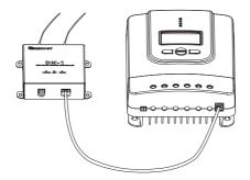
Step 3 Connect power cable to load terminals of the charge controller. If the controller doesn't have load terminals, alternatively connect power cable to battery terminals. However, for the best performance, it is suggested to connect power cable to load terminals.
