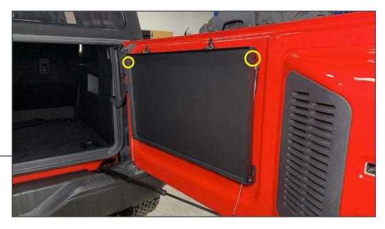
Secure the hanging straps to the bottom of the tray using (1) M6 x 15mm Allen bolt, (2) M6 flat washers, and (1) M6 lock nut per side.
