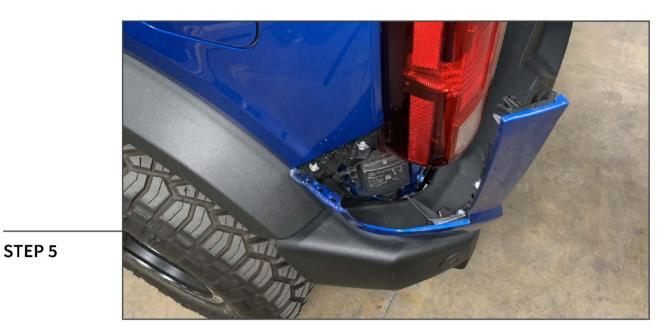
Pull outwards on the horizontal portion of the tail light trim, then pull upwards to remove the trim from the vehicle.
