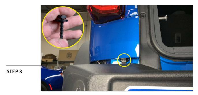
In between the vehicle body and the rear bumper, remove (1) 10mm bolt.
