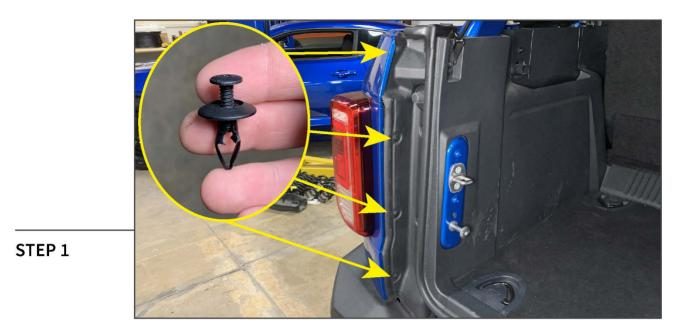
Remove (4) Phillips head plastic push clips. Loosen the Phillips head inner portion of the clip, then pull the plastic clip body out of the vehicle.
