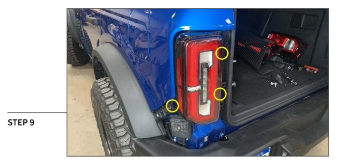
Plug in the new LED tail light, and secure to the vehicle using the original hardware.
