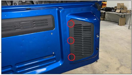
Open the vehicle tailgate, and remove the interior plastic trim panel using a panel removal tool.
