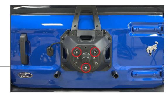
Remove the vehicle spare tire by removing the (3) lug nuts.
