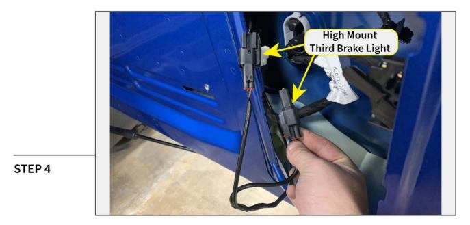
Locate the vehicle high mount third brake light wiring harness connector in the tailgate. Plug in the spare tire brake light 'T' harness into each end of the vehicle high mount third brake light wiring harness. Ensure each connector audibly clicks into place to ensure proper connection.
