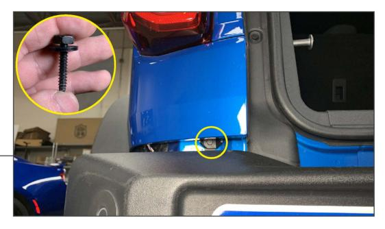
In between the vehicle body and the rear bumper, remove (1) 10mm bolt.
