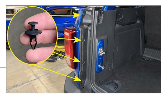
Remove (4) Phillips head plastic push clips. Loosen the Phillips head inner portion of the clip, then pull the plastic clip body out of the vehicle.
