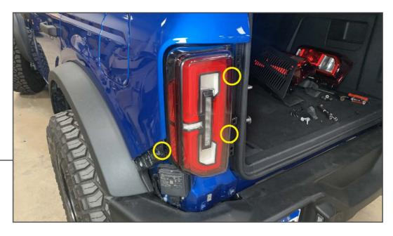
Plug in the new LED tail light, and secure to the vehicle using the original hardware.
