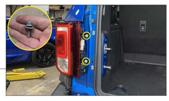
Remove (2) 8mm bolts from the inside of the tail light assembly. Firmly pull the tail light assembly away from the vehicle body to dislodge the alignment pin.
