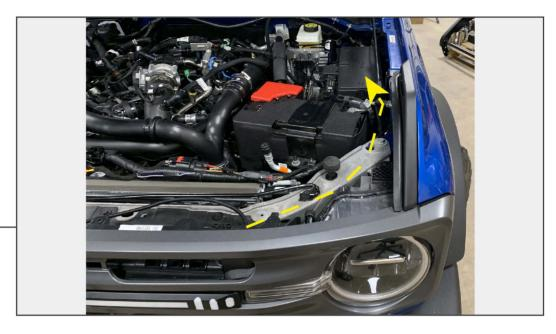
Neatly route the wiring harness along the back-side of the grille using the included wire retainers and foam adhesive pads. Ensure to avoid wire retainer placement around the grille mounting locations to prevent interference.
