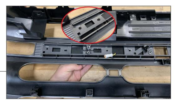
Place each light assembly onto the outside of the grille, and secure to the back of the grille using the provided (16) Phillips screws.
