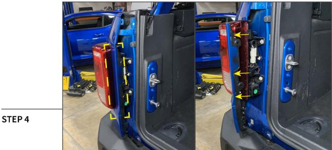
Using a plastic pry tool, pull the vertical section of the tail light trim outwards.
