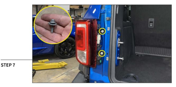
Remove (2) 8mm bolts from the inside of the tail light assembly. Firmly pull the tail light assembly away from the vehicle body to dislodge the alignment pin.
