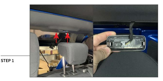
Using a pry tool, pry down on the sides of the rear dome light to gain access to the dome light harness. Unplug the wiring harness from the dome light.
