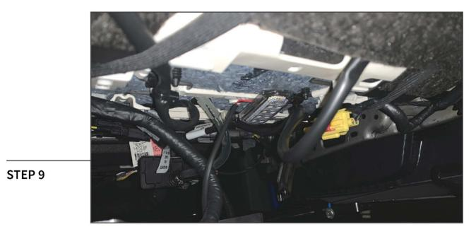
Under Seat Lighting: Plug in the LED light to the previously routed wiring harness. Then, attach the hooks on the LED lights to the under side of the seat.
