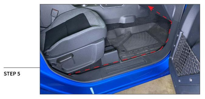
Pull upwards on the door entry trim panel and route the wiring harness under the vehicle trim. Route the wiring harness under the vehicle dashboard on both sides of the vehicle.
