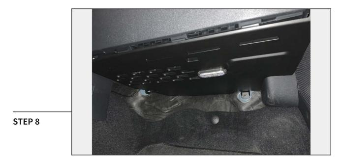
**Passenger Side Molle Panel:** Plug in the LED light to the previously routed wiring harness. Then, align the molle panel to the vehicle holes in the firewall. Secure the bottom mounts using (2) plastic push clips. Press the front of the molle panel upwards to fit flush with the dashboard.
