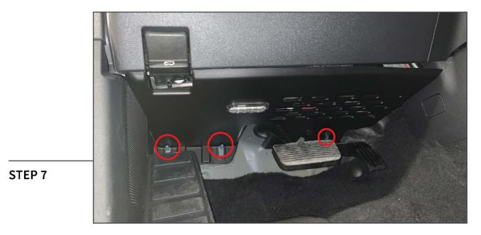
**Driver Side Molle Panel:** Plug in the LED light to the previously routed wiring harness. Then, fit the molle panel to the (3) studs in the vehicle firewall. Using the (3) provided nuts, secure the molle panel. Press the front of the molle panel upwards to fit flush with the dashboard.
