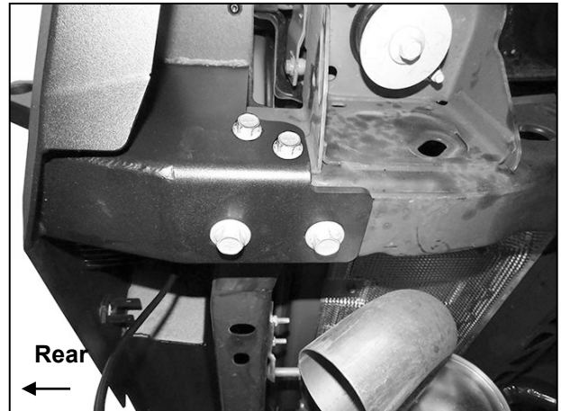
(Fig 14) Passenger/right side of Bumper attached to bottom of frame and Double Nut Plate inside of frame
