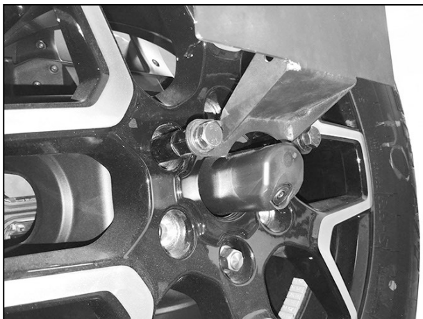
(Fig 19) Relocation Bracket installed
