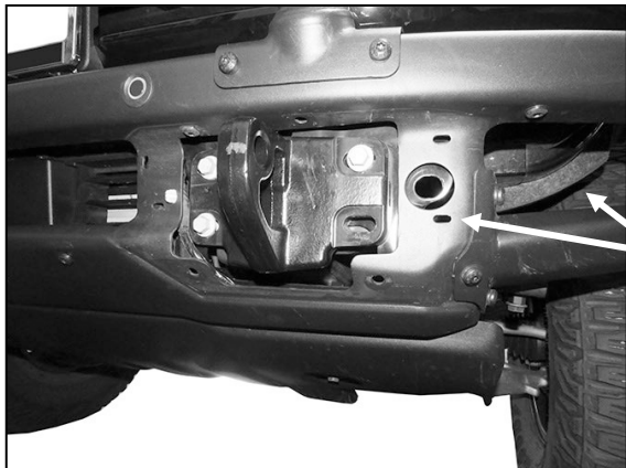
(Fig 3) Model with steel bumper, remove cover from bumper (driver/left side pictured)
