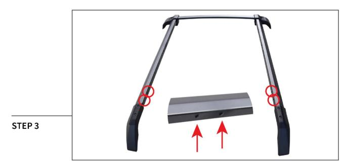
Remove the (4) plugs from the roof rack side rails.
