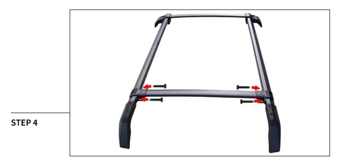
Place the accessory bar onto the roof rack, and secure into place using the (4) Torx bolts. Tighten until secure.
