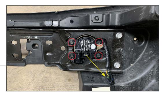
Unplug the fog light wiring harness from the fog light assembly. Remove (4) 10mm screws from the fog light. Remove the fog light from the bumper.
