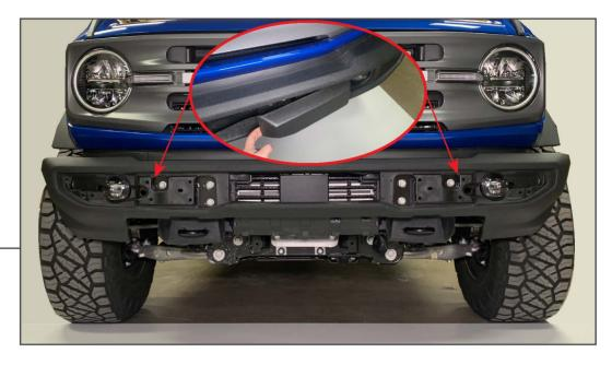
Remove the (2) plastic bumper covers using a plastic panel removal tool to reveal the bumper mounting hardware.
