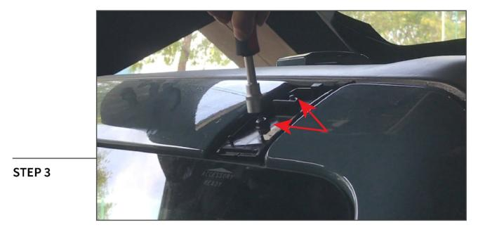
Remove the (2) 10mm nuts from the vehicle studs.
