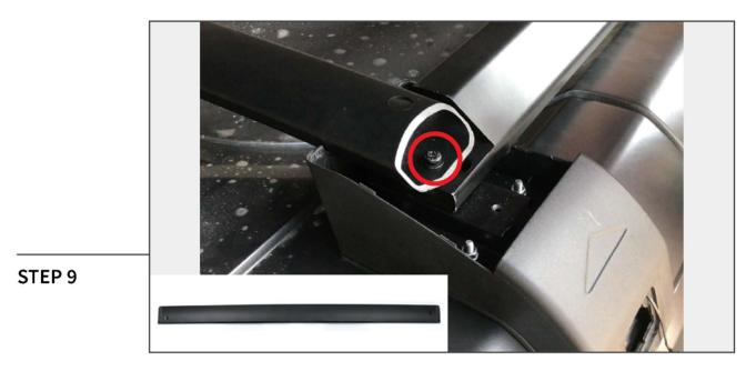
Secure the horizontal bars to the vertical bar/rear mounting brackets using (1) M6x1.00 Torx Bolt w/ Washer per side.
