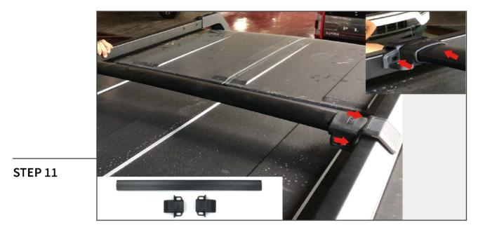
Insert the middle cross bar with the end caps, and secure to the roof rack using the provided hardware.
