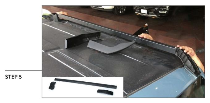
Fit the roof rack vertical bar with the appropriate front bracket to the windshield bar and align the front vehicle studs.
