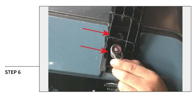
Secure the front mounting brackets using (2) provided M6x1.00 nut bolts.
