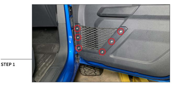
Remove (6) T-30 Torx bolts from the door panel.
