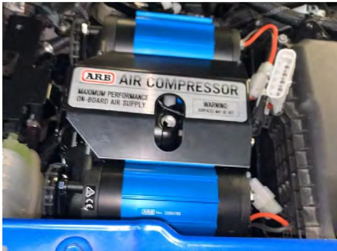
24. Carefully install the assembled Compressor, base plate and DLCM onto the support brackets.
