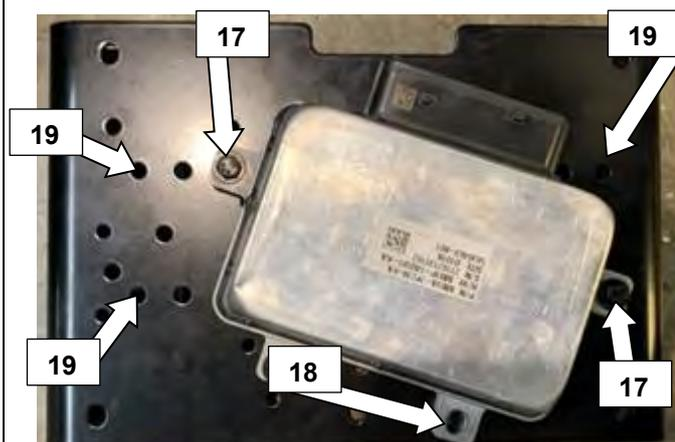
16. Place base plate onto the Compressor along with the DLCM.
