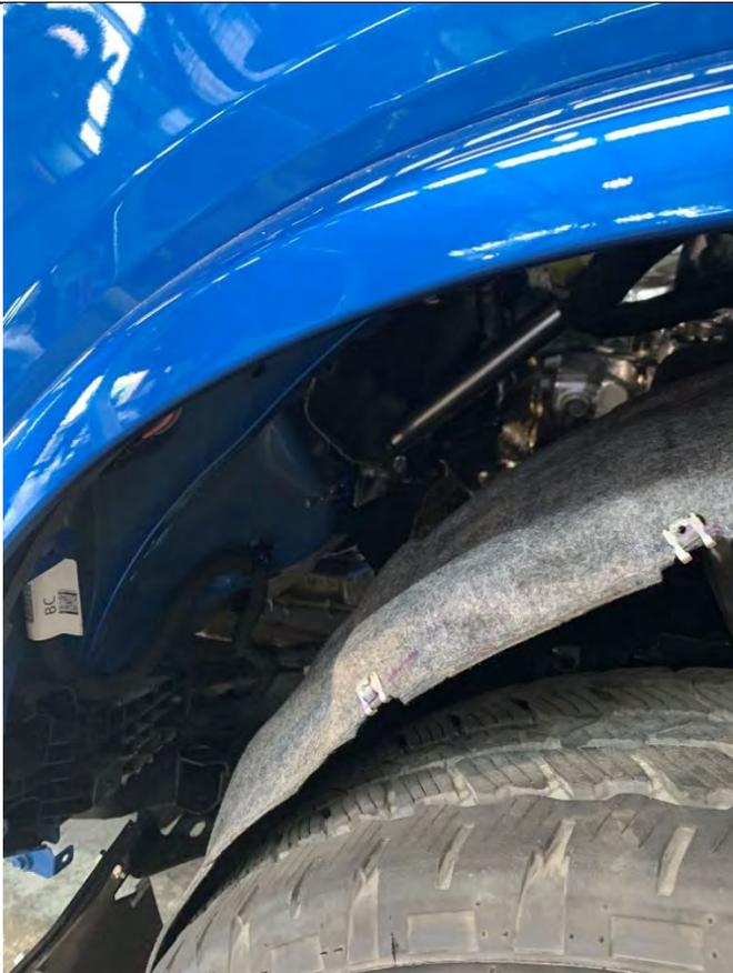
3. Remove fasteners (rear half only) for RHS inner guard and lower.
