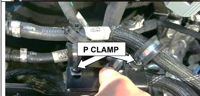
20. Secure the coolant hoses with two P clamps, M6x16mm bolts, washers, and flange nuts.
