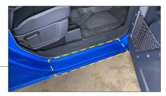
Using the designated door entry guard, test fit the guard to the vehicle before removing the adhesive tape. Once familiar with fitment, clean the vehicle using isopropyl and a microfiber cloth at the guard adhesion location.
