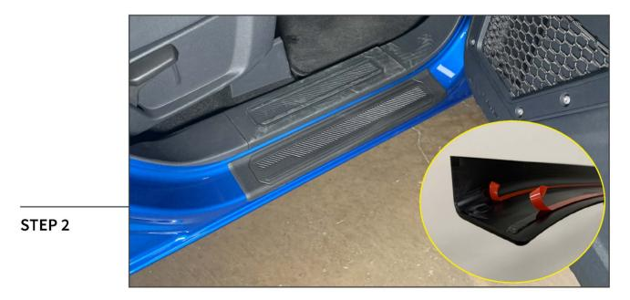
Peel the double sided tape backing, and adhere the entry guard to the vehicle. Press the entry guard down firmly to ensure proper adhesion.
