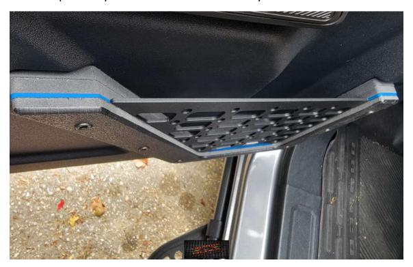
5. Repeat steps 1-4 for the other door. The PSD net will leave 3 to 4 inches between the door and seat for Molle pouches for storage.
