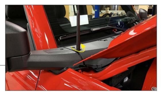
Twist the vehicle antenna counter clockwise to unthread the antenna from the vehicle cowl.
