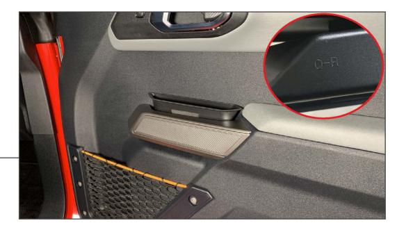
Identify each door panel storage pocket using the embossed identifier on the bottom of the pocket. Once identified, locate the vehicle interior door grab handle and place the pocket into the door.
