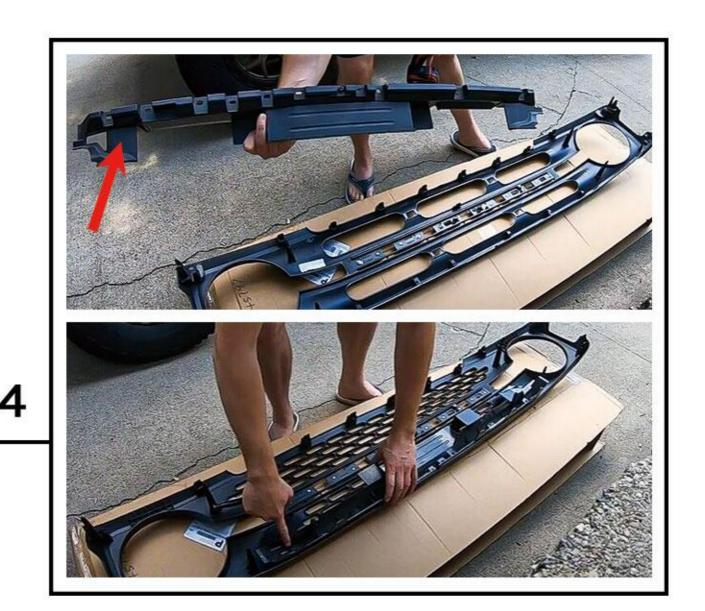
Remove this bracket from the original grille and transfer it to the new grille.
