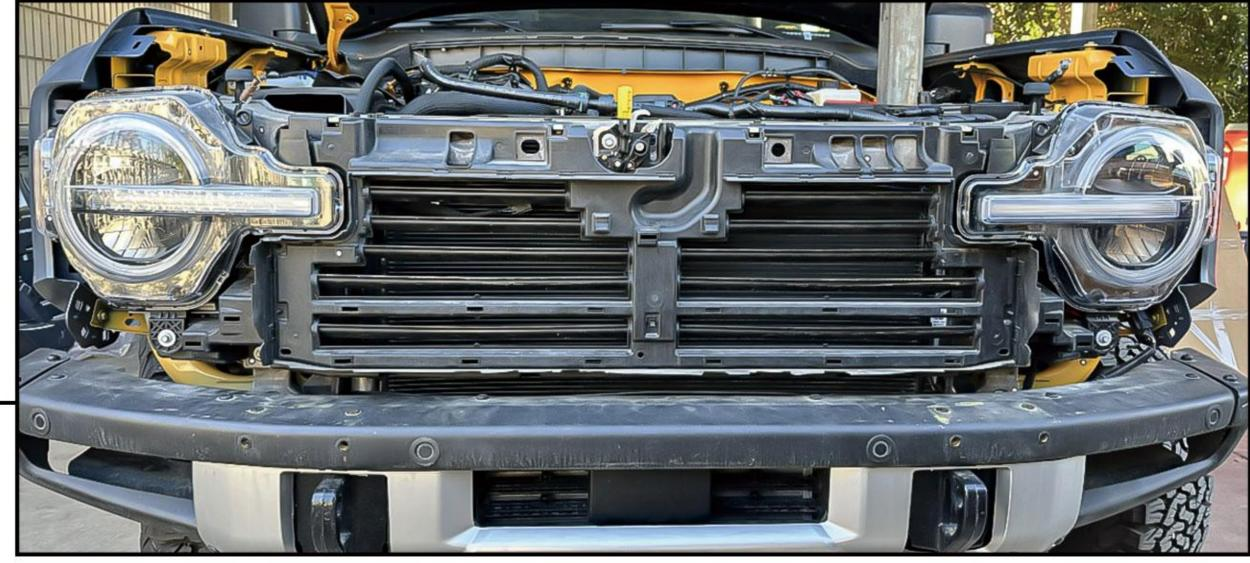
Remove the 8 clips and remove the cover panel. Remove the 4 screws. Unplug the wire harness and pull the original grille from the vehicle.
