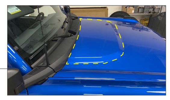
Clean the hood bulge perimeter using the (2) adhesion promoter prep pads. Allow the adhesion promoter to fully dry. Test fit the hood scoop to the vehicle hood prior to peeling the double sided tape backing.
