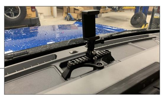
Adjust the phone mount to the optimal mounting position, then tighten all of the phone mounting assembly hardware.
