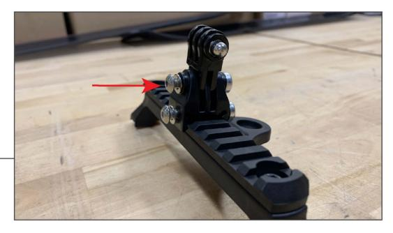
Install the upper adjustment bracket to the lower adjustment bracket. Begin threading, but do not tighten the upper mounting Allen bolt.
