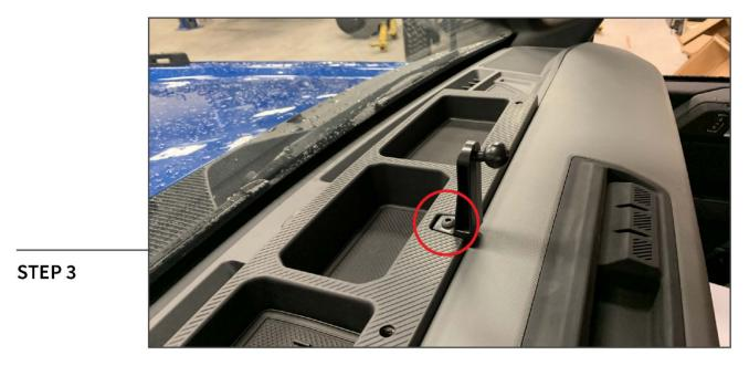
Align the (1) mounting arm to the front of the organizer, and secure the mounting arm into place using the provided (1) 1/4 - 20 Allen bolt. Tighten the bolt until secure.
