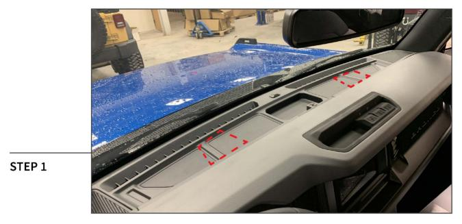
Clean the highlighted areas of the vehicle dashboard using isopropyl alcohol and a microfiber cloth. Allow to fully dry.
