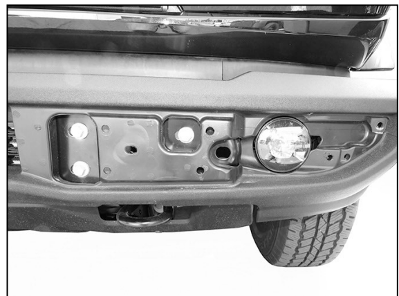
(Fig 2) Models with plastic bumper cover (see Fig 1), remove bumper pads from bumper (driver/left side pictured). Note, unplug parking sensors if equipped
