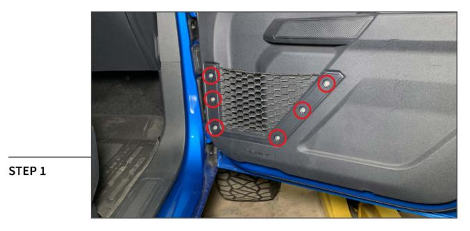
Remove (6) T-30 Torx bolts from the door panel. Remove the panel with netting from the vehicle.
