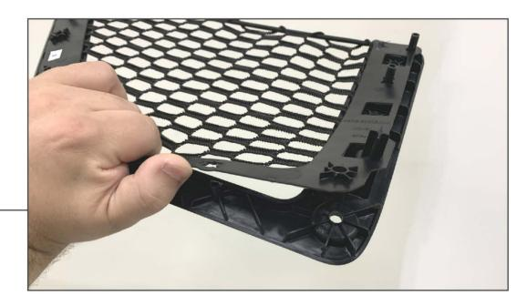
Separate the netting layer from the vehicle panel.
