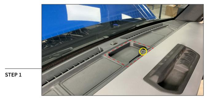
Clean the center dashboard cutout of all contents. Locate the (1) bolt hole in the dashboard.
