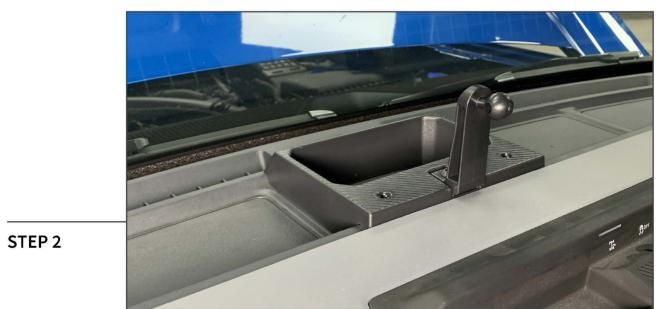
Place the storage organizer into the dashboard cutout. With the phone mounting post in place, secure the organizer and the post to the vehicle using (1) 1/4-20 Allen bolt. Tighten until secure.
