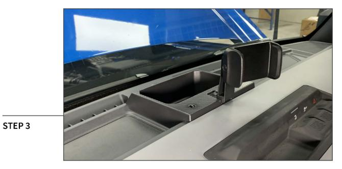
Install the phone clamp nut onto the post, then clip the clamp onto the post assembly. Secure the clamp using the previously placed nut. Tighten the phone clamp while having the clamp angled at the final resting position.
