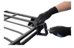
Place the Holding plate (B) on the rear of the side and insert the bolts (D) with washers (E) thorugh the holes and then place the washers (E) and nylon loc knuts (F). See the top image as reference.
