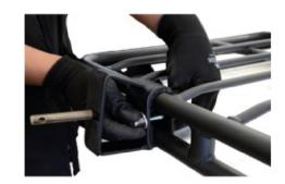
Tighten the all hardware using a 9/16" wrench and 9/16" ratchet tool.
