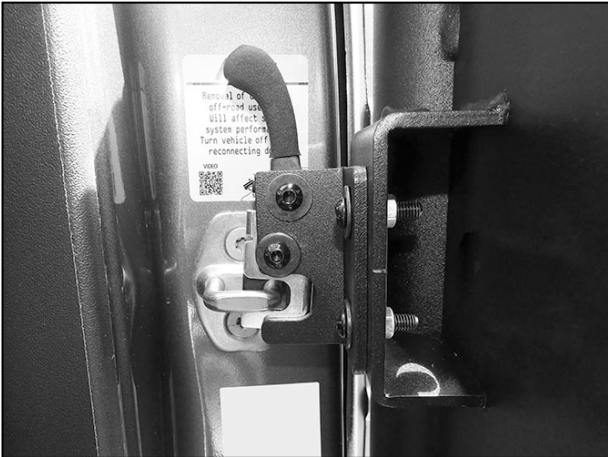
(Fig 14) Adjust Door and Latch assembly for proper operation before fully tightening hardware. Make sure door latch fully closes against striker
