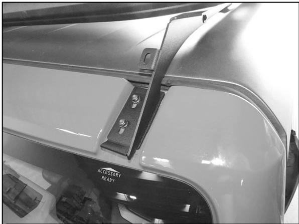
(Fig 17) Attach front mounts to threaded studs and Shims above front windshield
