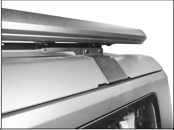
(Fig 18) Hook Outer Clamp Bracket into slot above rear side windows
