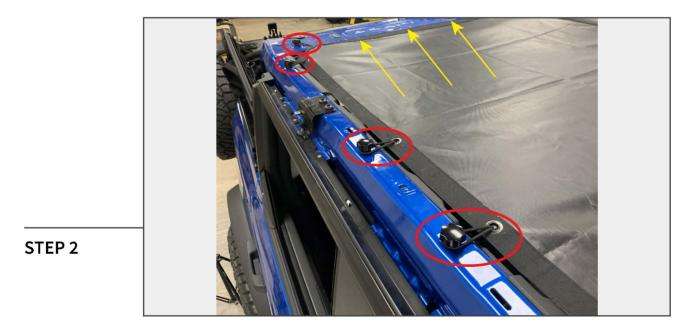
Align the sun shade to the vehicle. Install the (4) M8 thumb screws into the threaded holes in the roll bar on each side. Once threaded, secure the sun shade to the thumb screws using (4) elastic bands on each side.
