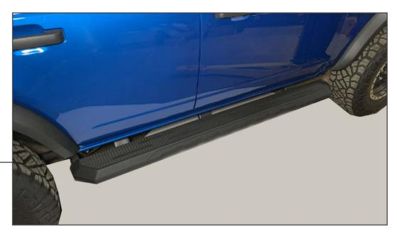
Adjust the mounting bracket to the ideal mounting location within the brackets. Tighten all hardware until secure. Repeat steps 1-3 to the opposite side of the vehicle.
