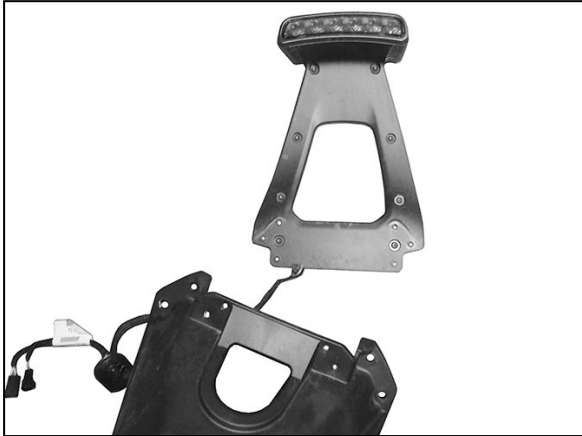
(Fig 19) Remove the brake light assembly from the top of the spare tire mount
