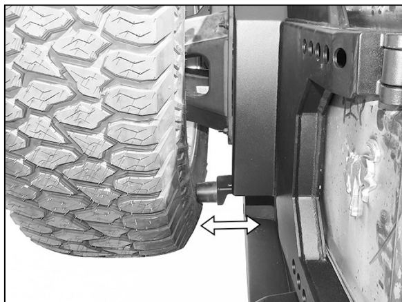
(Fig 23) Adjust rubber bumpers in or out to support the spare tire
