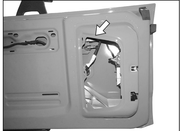
(Fig 2) Disconnect wire harnesses leading to the camera and CHMSL (3rd brake light). Release rubber grommet and pull outer harness through hole in rear door.
