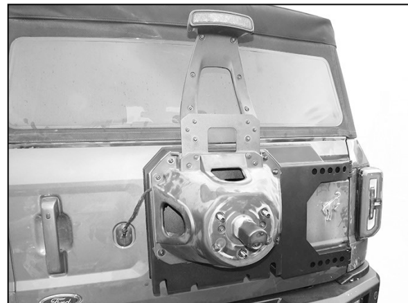
(Fig 22) Attach the factory spare tire mount to the Tire Carrier, (also see Fig 21)
