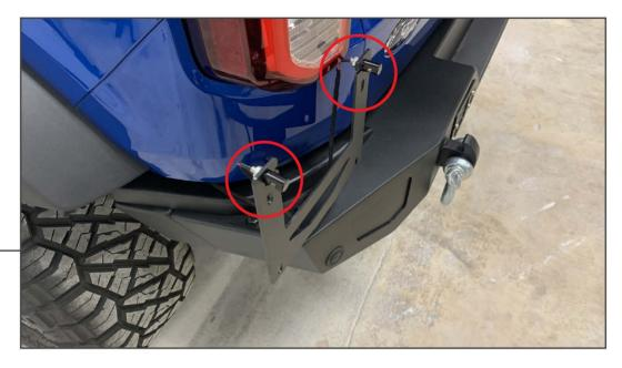
Install the LED license plate bolts to the license plate bracket using the pre-installed hardware. Plug the harness connector into the vehicle license plate wiring harness.
