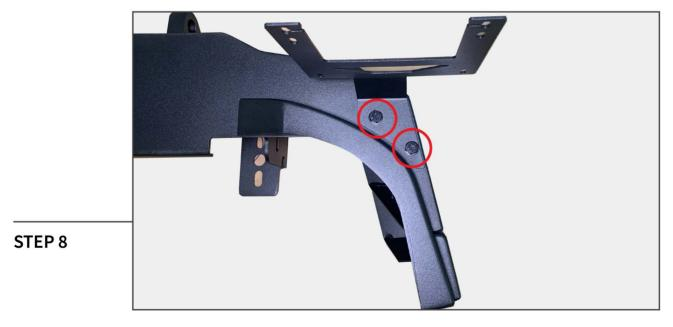
Secure the license plate mounting bracket to the bumper using (2) M10 x 25mm bolts, (2) M10 flat washers, (2) M10 lock washers, and (2) M10 flange nuts.
