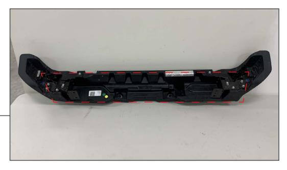
Unplug the license plate light and backup sensor harness from the bumper. Using a panel removal tool, remove all the wiring harness retaining push pins to remove the harness from the bumper.
