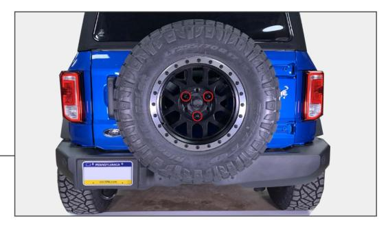
Remove the (3) lug nuts from the spare tire and remove the spare tire from the vehicle.
