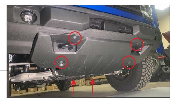
Remove (6) 15mm bolts from the lower splash shield.
