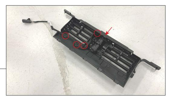
Unplug the shutter assembly motor by sliding the red lock, and pressing the tab. Then, use a pry tool to dislodge the wiring harness from the shutter assembly. With the harness removed, mount the shutter assembly to the vehicle using the original (4) 8mm bolts.
