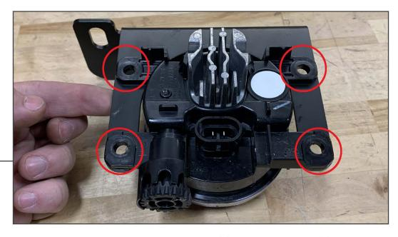
Secure each fog light to the included mounting bracket using (4) M6 x 20mm bolts, (8) M6 flat washers, (4) M6 lock washers, and (4) M6 nuts. Tighten until secure.
