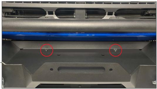
Install the rear block off plate to the bumper. Plate the panel under the bumper winch plate surface, and secure using (2) M8 x 30mm bolts, (2) M8 flat washers, and (2) M8 flange nuts.
