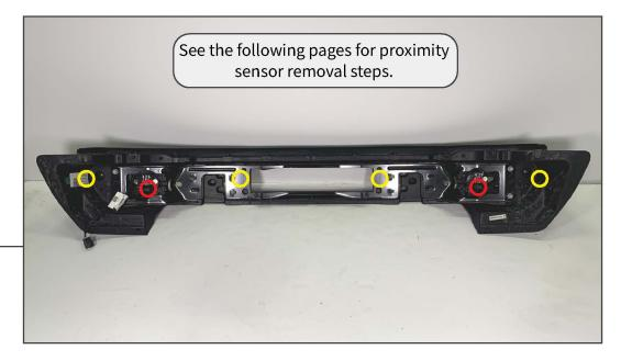
Unplug the wiring harness from each fog light and proximity sensor. The proximity sensors can be used on the new bumper.
