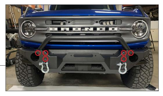
Place the (2) bumper mounting nut plates behind the vehicle frame rails. With assistance, install the bumper to the vehicle frame rails using (6) M12 x 50mm bolts, (6) M12 flat washers, and (6) M12 lock washers. Do not fully tighten to allow for adjustment later.
