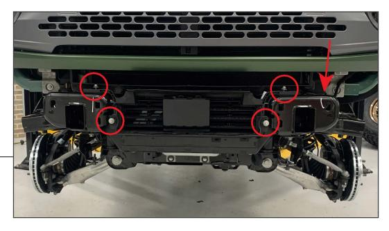
With the bumper removed, locate the front lower shutter assembly. Unplug the wiring harness connector along the LH side of the vehicle, and remove (4) 8mm bolts from the shutter assembly. Remove the shutter assembly from the vehicle and place on a workable surface.
